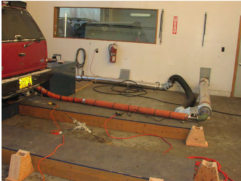
Figure 3-1 Mixing Chamber, Dilution Tunnel, and Heated Transfer Tube
