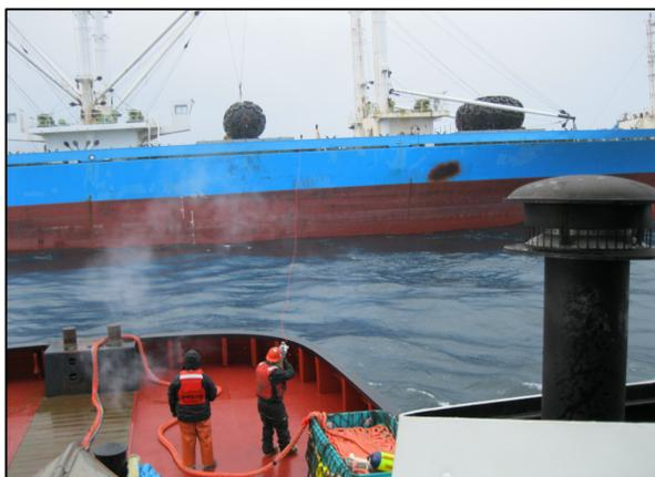
Photo 2: GYRFALCON delivers ETS messenger via line throwing gun
