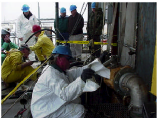
Testing in progress, MMS OHMSETT employee (foreground) records system pressure as ESSM and USCG Personnel (background) operate and record system flow rate and hydraulic controls while pumping oil with ESSM pump systems. Ohmsett, NJ, March 2000.
