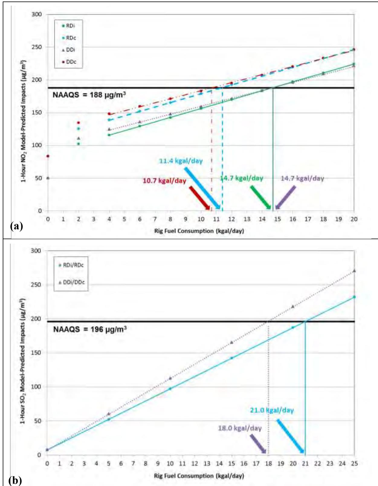
**Figure 10 (a) 1-hour NO<sub>2</sub> and (b) 1-hour SO<sub>2</sub> Model-Predicted Impacts after TRANSVAP Post-Processing**
