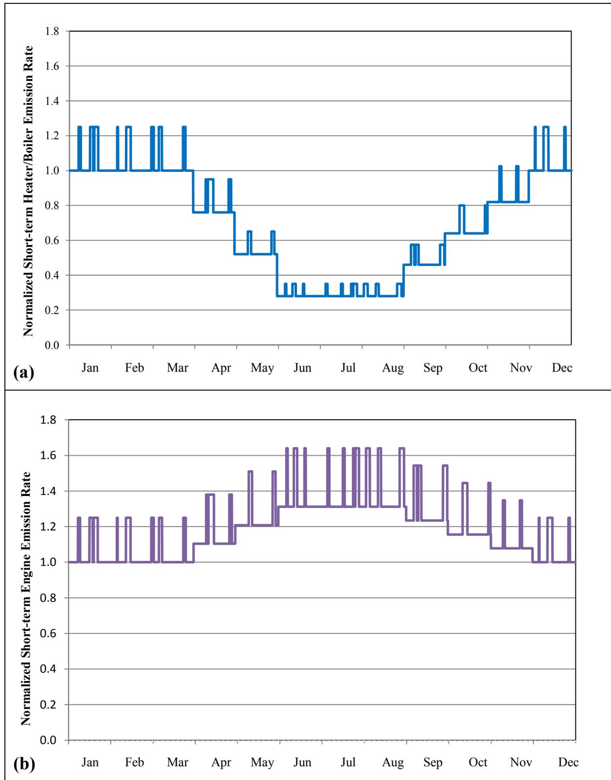
**Figure 5 Normalized 1-hour NO<sub>2</sub> Seasonally-Varying Emission Rates with Transient Hourly Excursions for (a) Heaters and Boilers and (b) Engines for a Typical Year**
