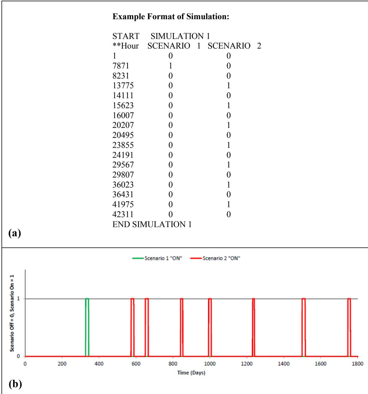
**Figure C2 Example (a) TRANSVAP Simulation File and (b) Graphical Depiction for a Single Simulation**
