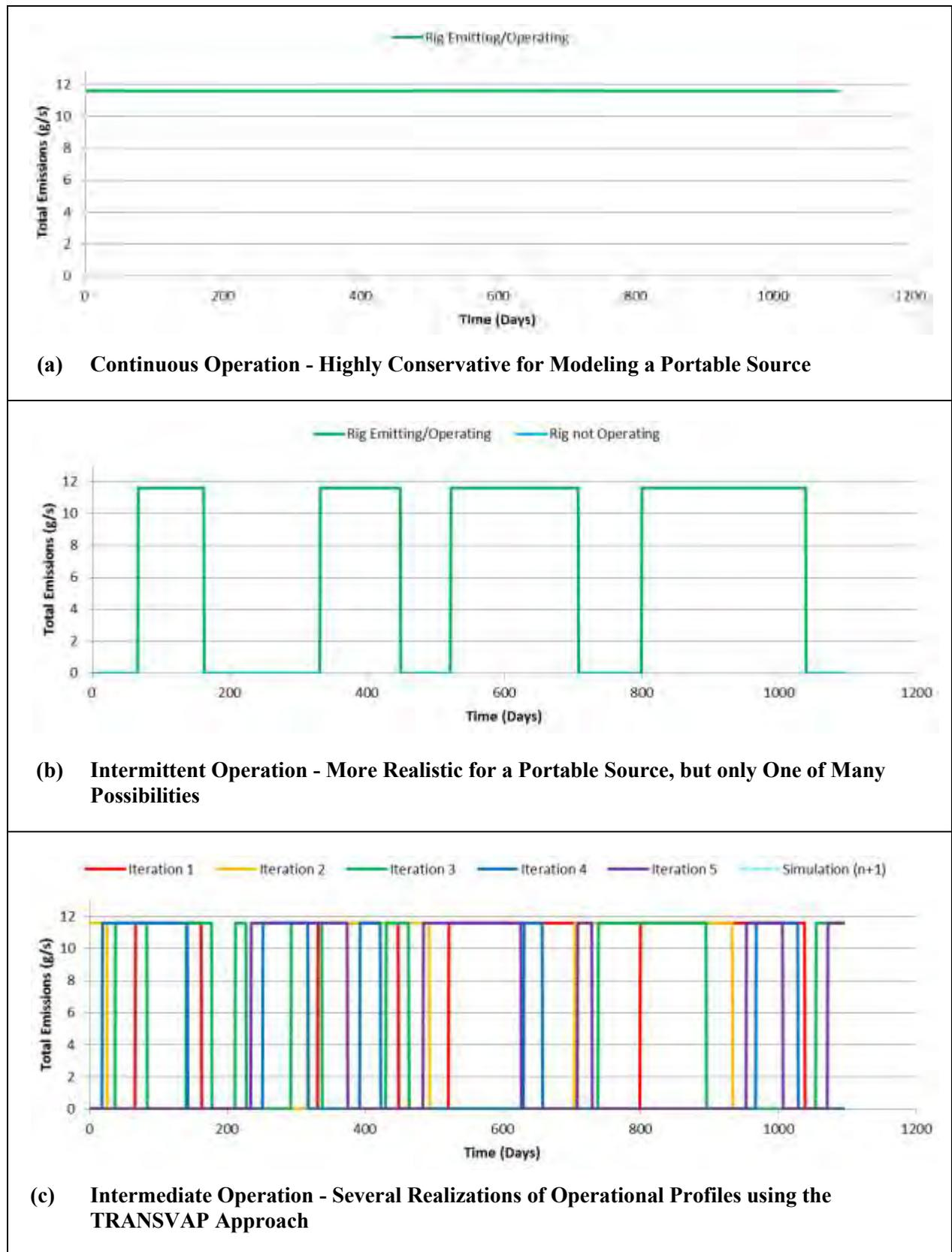
Figure C1 Potential Modeling Approaches for a Portable and Transitory Operation
