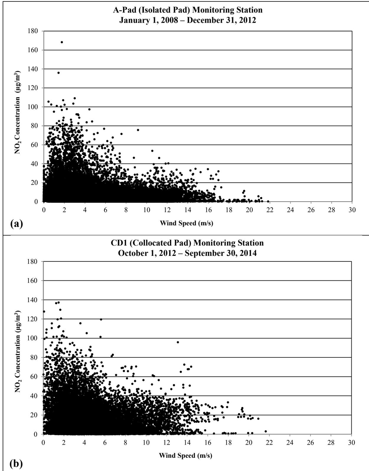
**Figure D1 Relationship Between Hourly NO<sub>2</sub> Concentrations and Wind Speed Measured at the (a) A-Pad and (b) CD1 Monitoring Stations**
