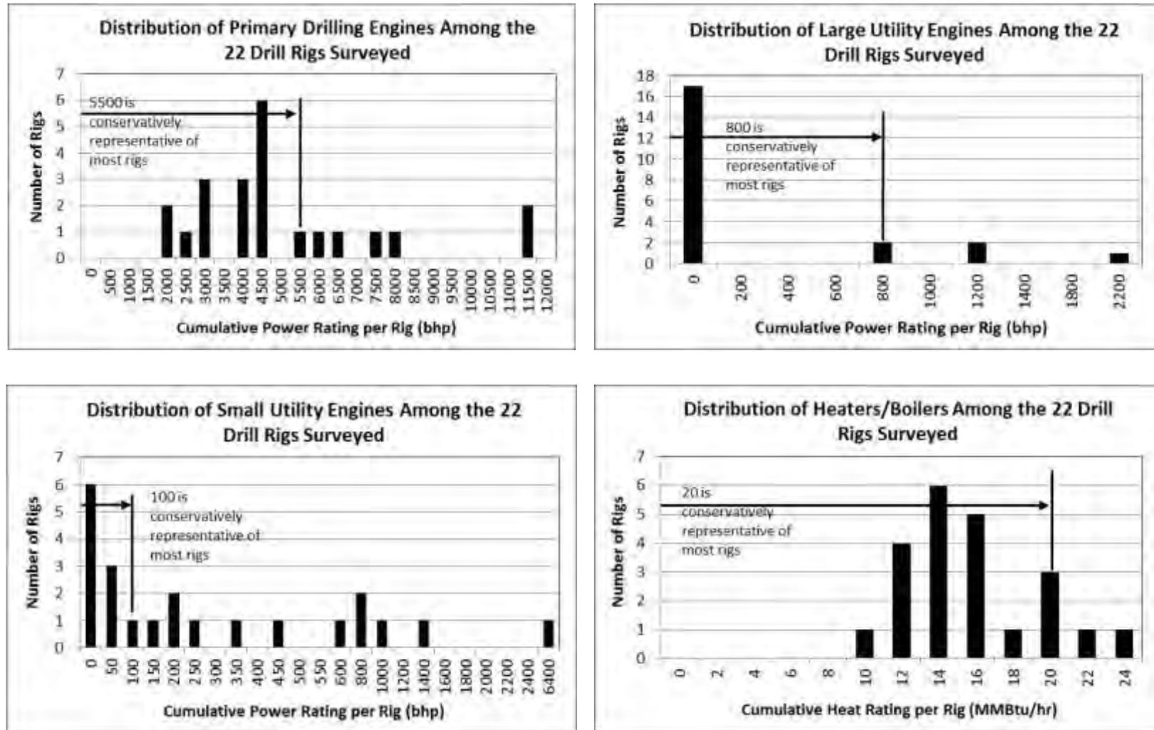
Figure B1 Results of Drill Rig Inventory Survey
