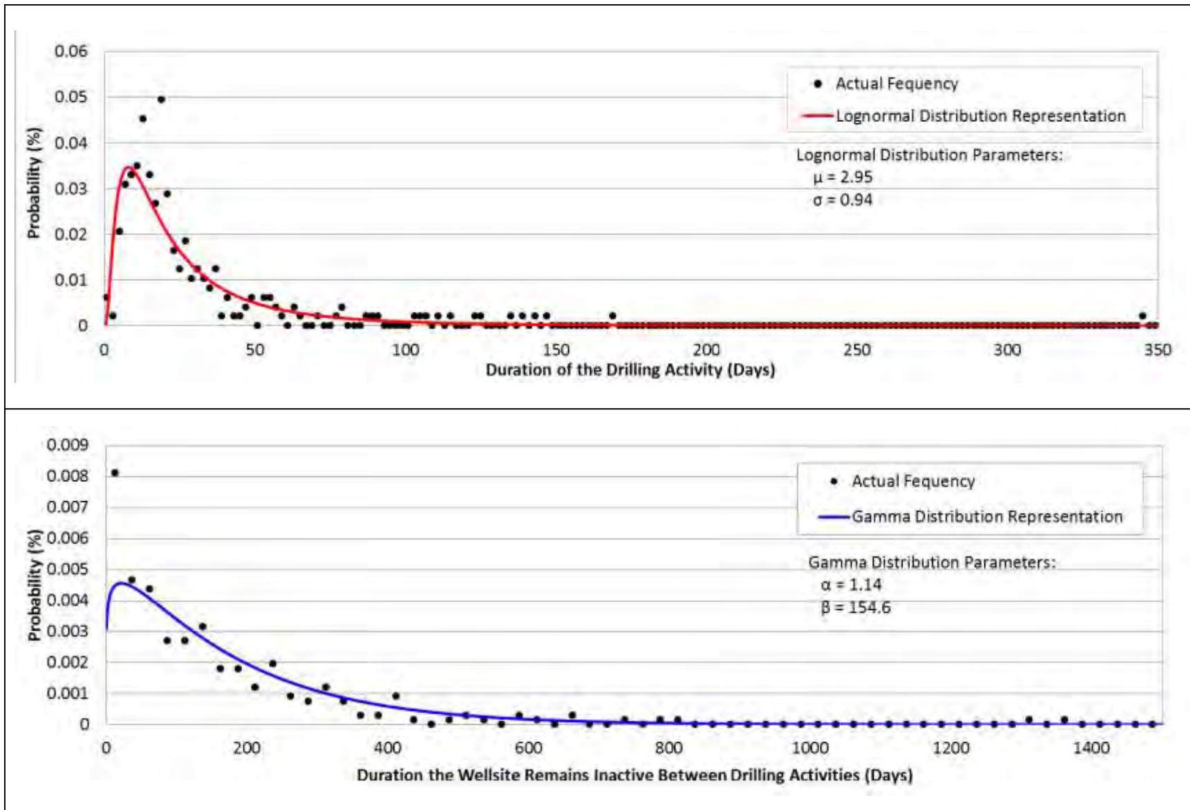
Figure C4 Representative Routine Infill Drilling Activity Profiles
