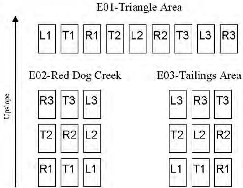
Figure 2. Ameliorative treatment plot layout in each experimental area. The treatments include lime application (L), triple superphosphate application (T), and untreated, reference (R) plots. E01 was set up in a single row because the slope length was insufficient to accommodate placing plots in multiple rows.
