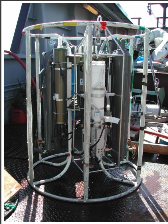
The field crew deploys the CTD and Niskin Rosette assembly. DEC photos.
