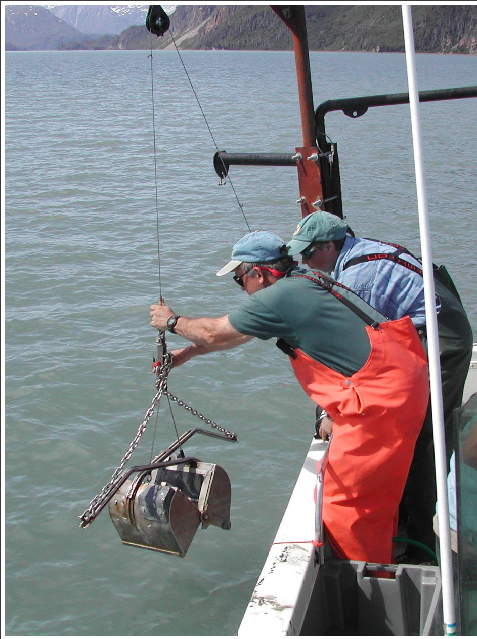
The field crew collects sediment samples with Van Veen sampler. DEC photos.
