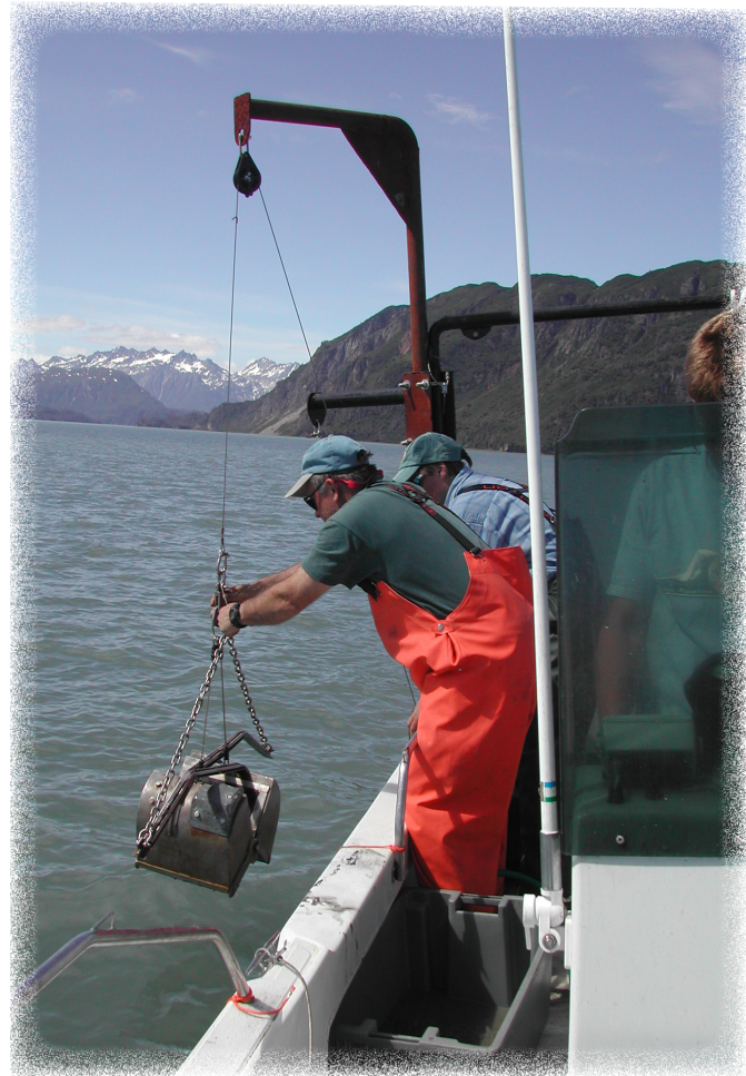
EMAP Crew member retrieves a Young-modified VanVeen grab with a sediment sample.
