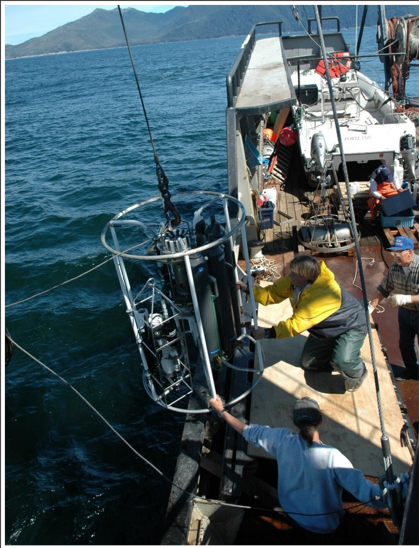
Crew members collect water and sediment samples using CTD and Van Veen samplers
