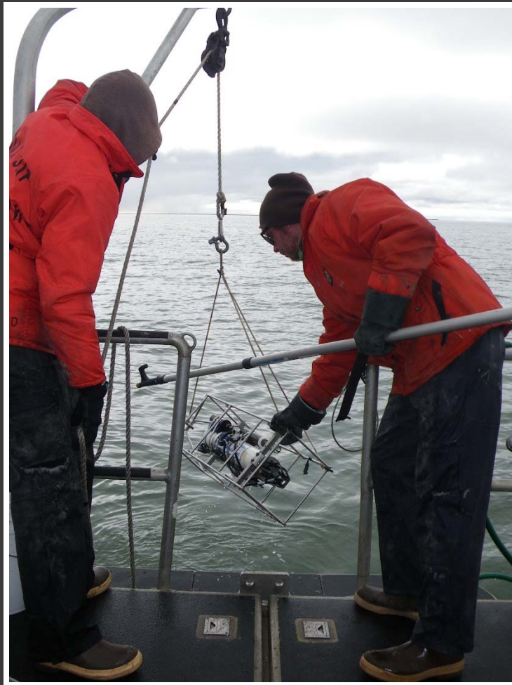
In situ water quality was analyzed using a Seabird 19plus.
