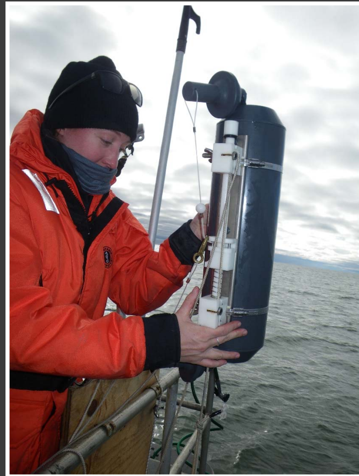
Water samples were taken using Niskin bottles.
