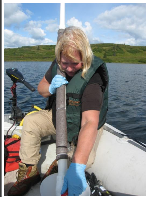
Obtaining water chemistry samples with Integrated Sampler.
