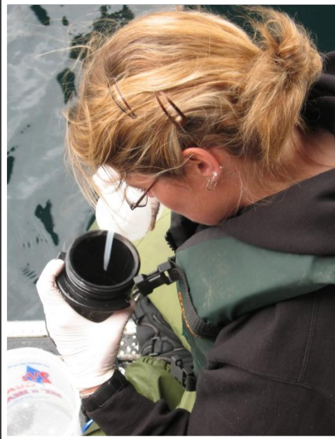
Washing down plankton in Plankton Net Collection Cup.
