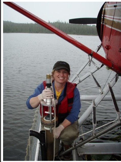
Sediment sample obtained with Sediment Corer.
