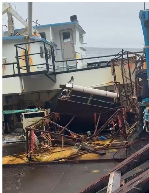
June 20, 2026, Sorting table crushed/blocking engine room access; Photo credit: Resolve Marine
