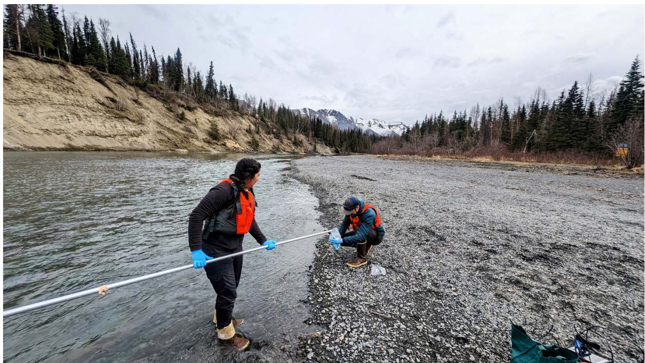
Figure 6. Water Quality Program staff use a dipper pole to collect water samples at the Eagle River Greenbelt site.
