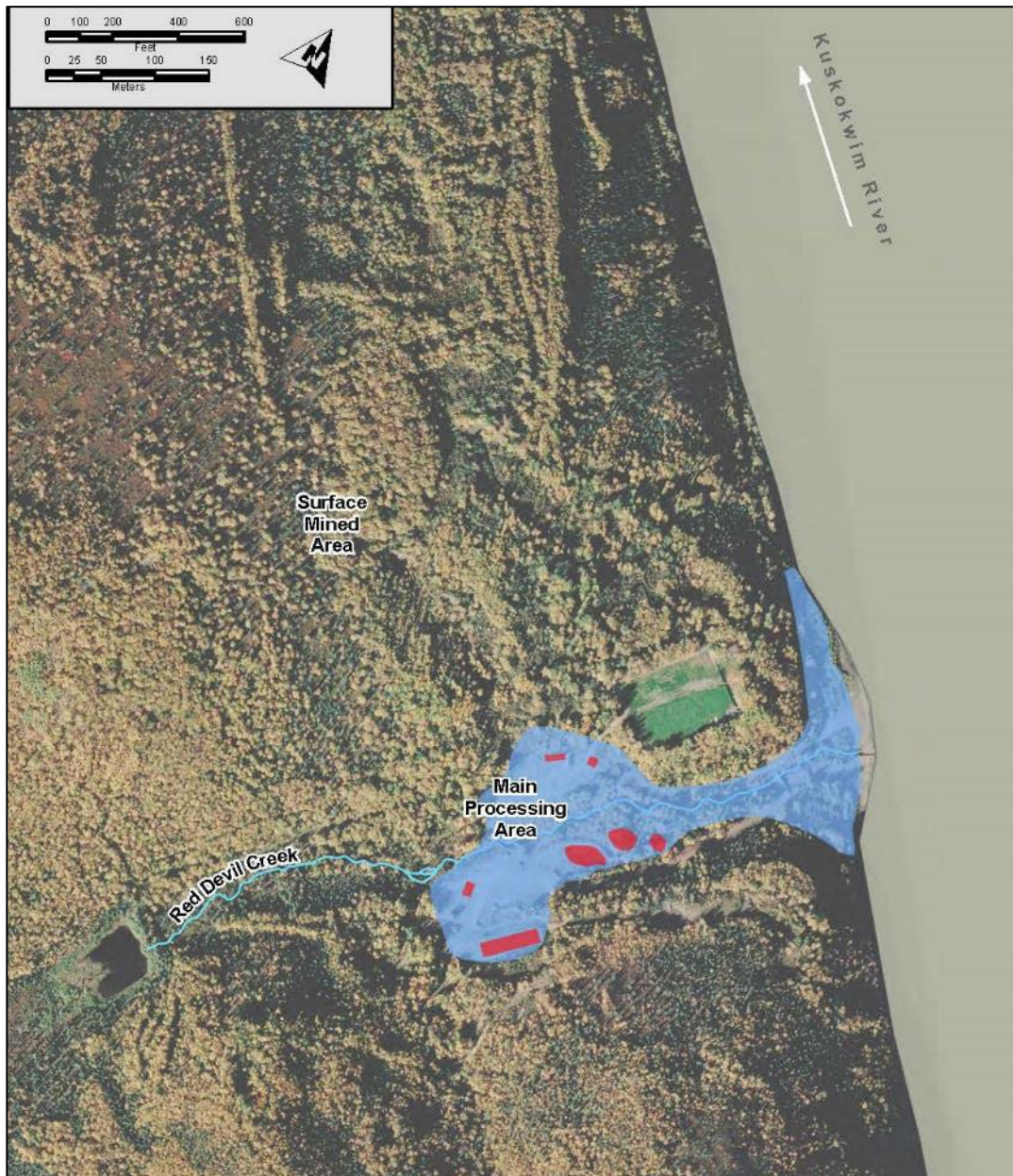
Figure 2. Map of site features at the historic Red Devil Mine. 5 The blue shading indicates areas impacted by tailings, waste rock and contaminated soil. The red shading shows ore processing waste source locations.
