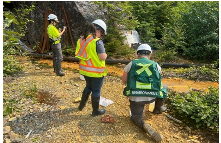
Discharge sampling being conducted at the 5400 portal
