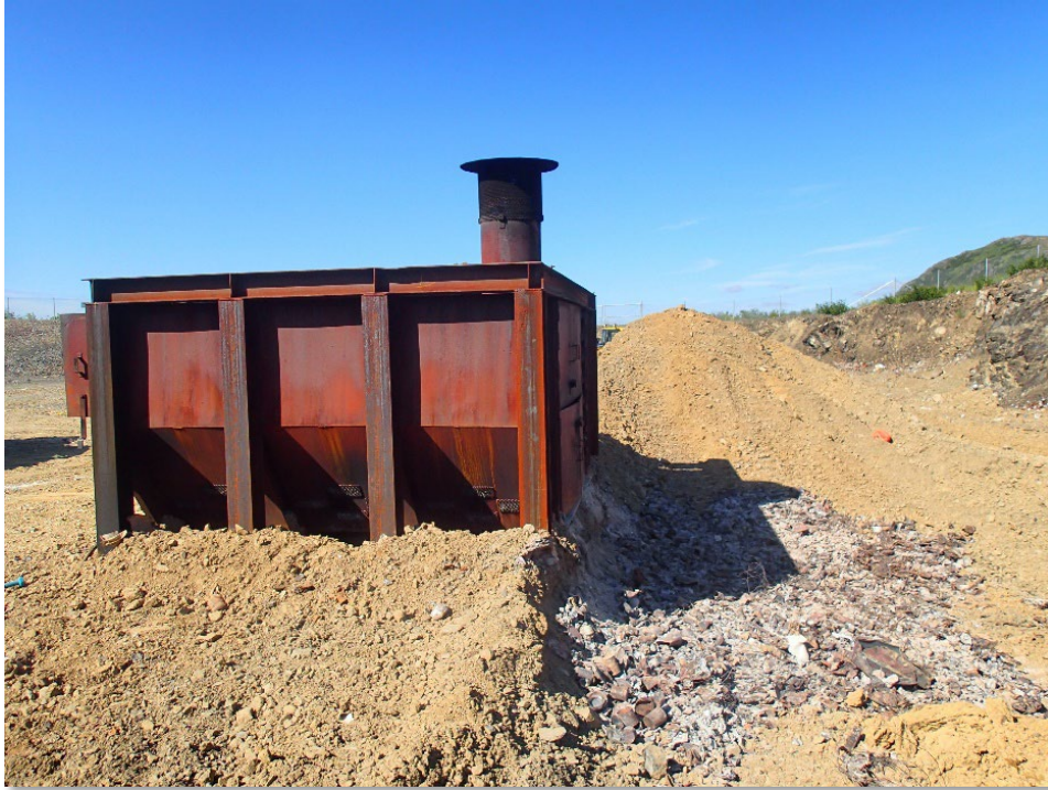
Enclosed commercial burn unit.
