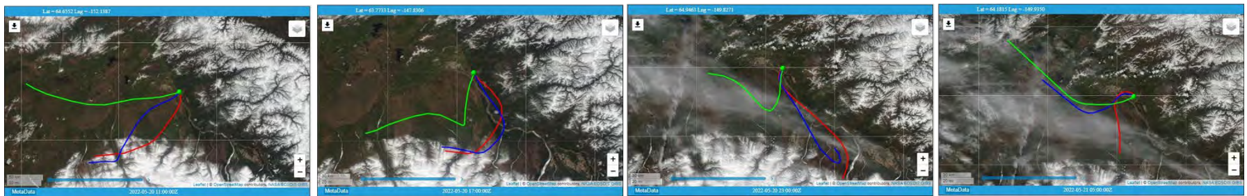
Figure 15: MODIS Imagery with HYSPLIT Overlay. Air parcel backward trajectories are shown at 100m AGL (red), 300m AGL (blue), and 1000m AGL (green).
