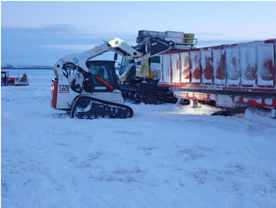
Figure 5. Loading contaminated snow into a bin for transport to Deadhorse on January 17, 2024. Photo provided by Alaska Department of Environmental Conservation.
