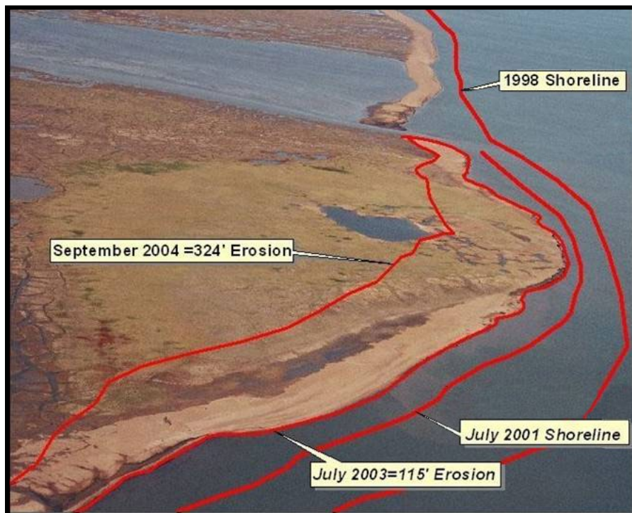
Figure 9-1: Drill Site Erosion
