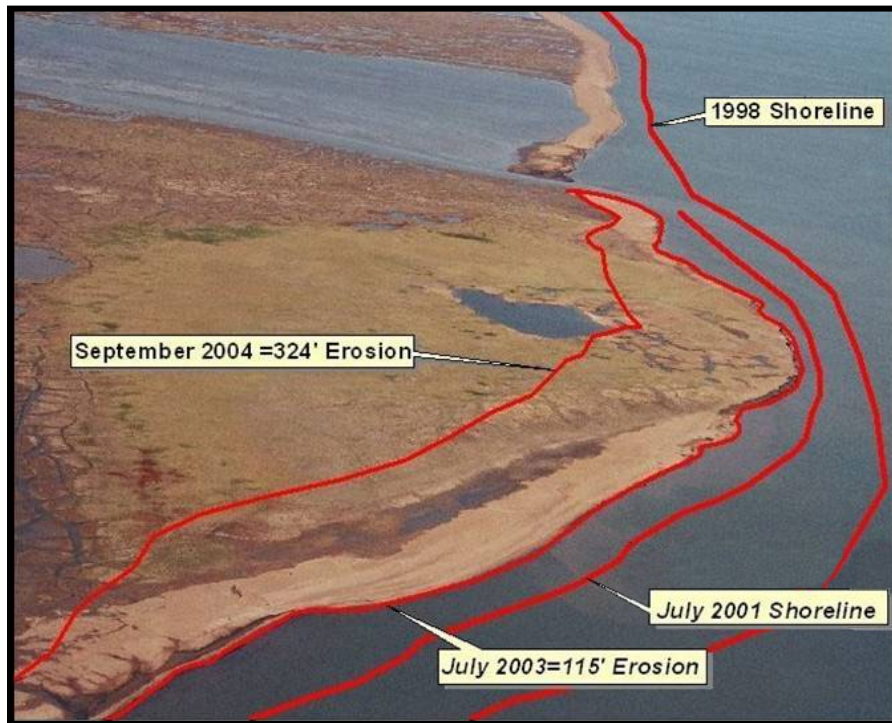
J.W. Dalton Drill Site Erosion. Located east of Utqiagvik on the Beaufort Sea near Teshekpuk Lake and Point Lonely DEW line site. This photograph was taken in 2003; between the summers of 2003 and 2004 over 300 feet of shoreline eroded away along part of the site. Approximately 600 feet of coastal plain were lost over a 6-year period. Photo provided by BLM
