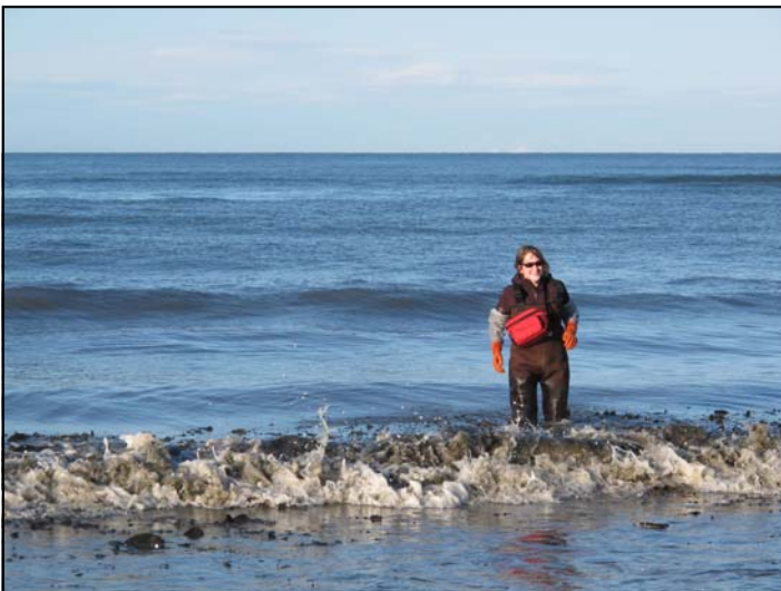
Figure 4. Inletkeeper intern Marcella Dent returns from sampling at Mariner Park. Sampling is done in approximately 3 feet of water, and samples are collected 1 foot below the surface.
