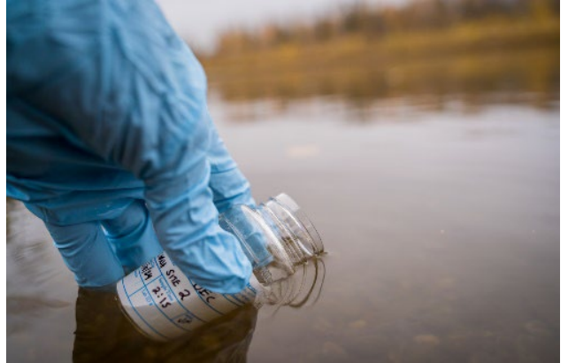
A sample bottle is dipped into the Chena River to collect a pathogen water sample. Photo by DEC staff Jeff Fisher
