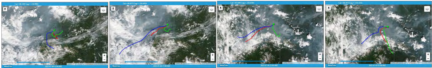
Figure 75: MODIS Imagery with HYSPLIT Overlay. Air parcel backward trajectories are shown at 100m AGL (red), 300m AGL (blue), and 1000m AGL (green).
