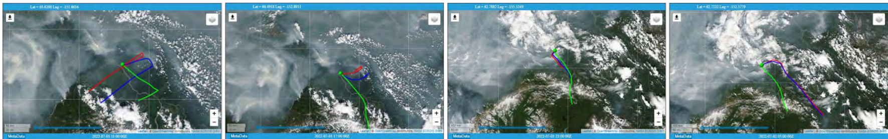
Figure 66: MODIS Imagery with HYSPLIT Overlay. Air parcel backward trajectories are shown at 100m AGL (red), 300m AGL (blue), and 1000m AGL (green).
