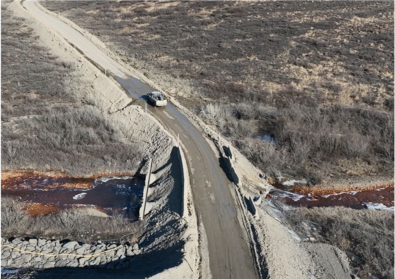
Figure 1: Image showing extent of the release along the road at the Red Dog Creek crossing. The area where the release breached the berm is to the left of the truck. Photo taken by Teck on May 14, 2025.
