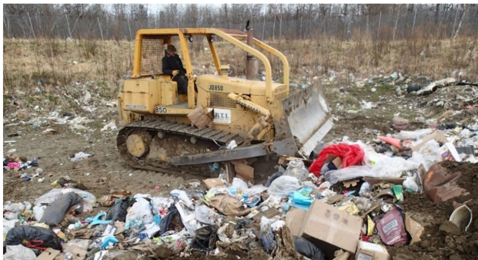
Operator using a dozer to consolidate waste.
