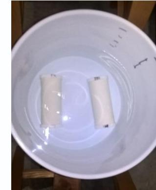
Dual filters with GAC packing achieved 100% chlorine removal
