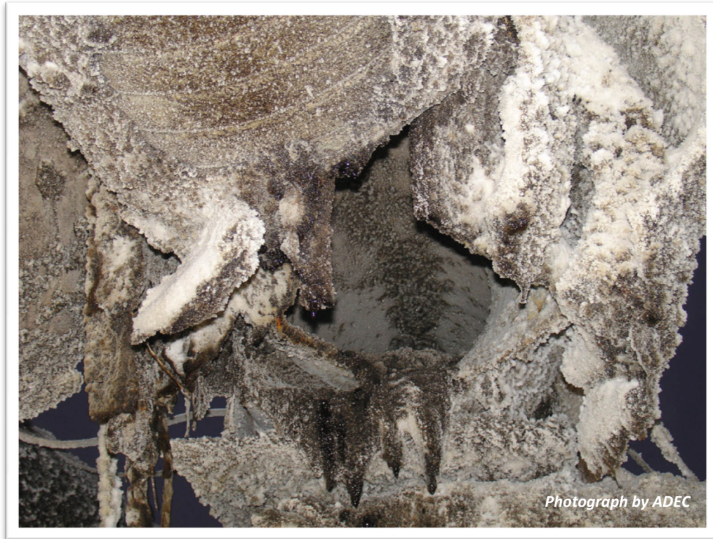
Rupture of the 18-inch pipeline.
