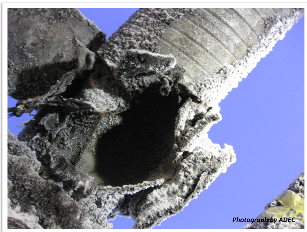
Looking up at the ruptured 18-inch pipeline.
