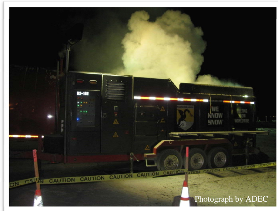
Snow melter melting down contaminated snow.
