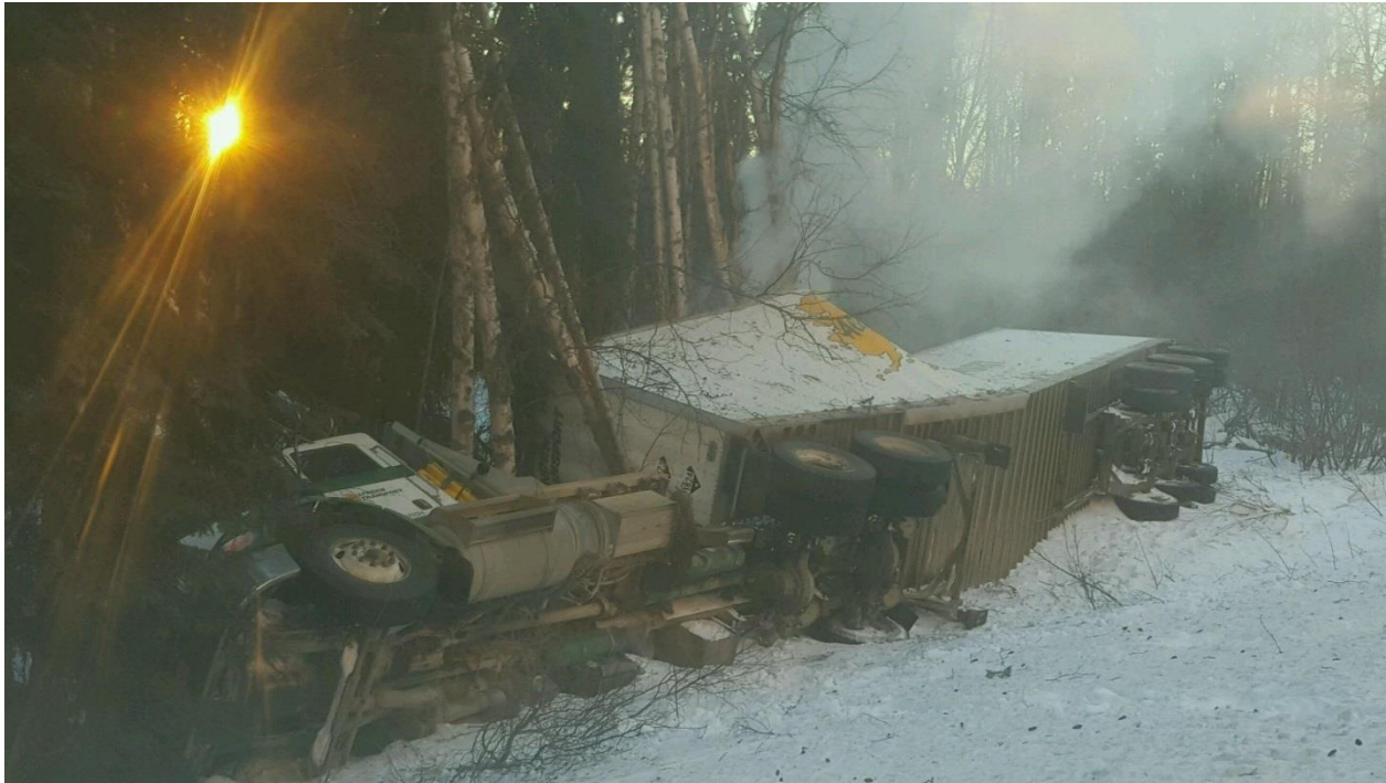
Figure 2. Lynden tractor and trailer on its side, off the roadway. The trailer has split and the white vapor emitting from the rupture is likely due to a chemical reaction. [Photo: NRC Alaska]
